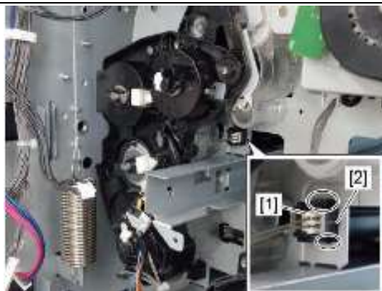
4、从后侧断开一处线束[1],松开两处卡扣,从前侧取下第二纸盒检测开关[2]
