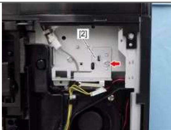
3、拧下一颗螺丝并拆下前盖板连锁开关支架[2]
