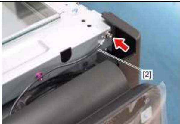
3、拧下一颗螺丝并取下接地线束[2]
