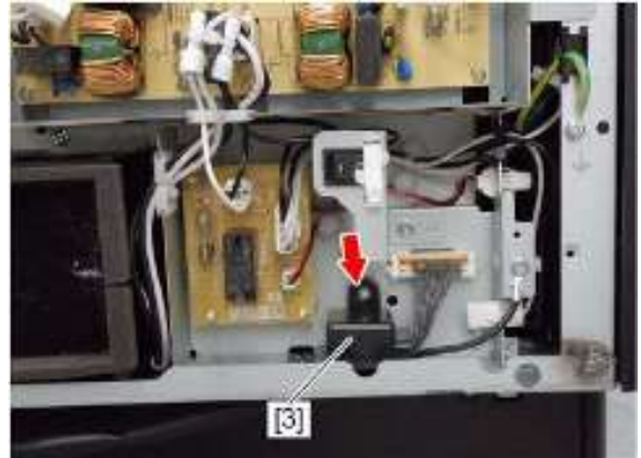
5、拧下 1 颗螺丝并拆下盖板[3]
